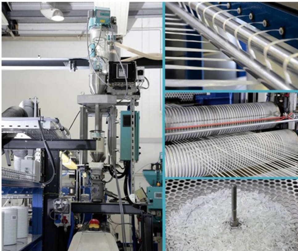
ProTec's LFT Pultrusion Lines are Suitable for Producing High Quality Long-fibre-reinforced Pellets with Many Different Polymer Matrices and Variable Fibre Reinforcement
